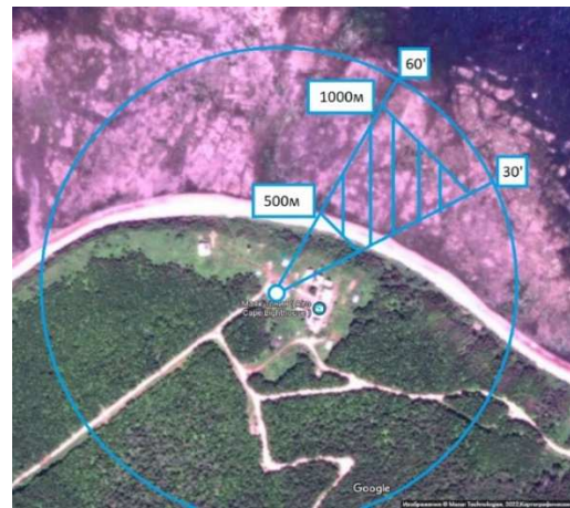
Fig. 1. Ray tracing scheme of the Mikran “River” RLS during the experiment conducted in Cape Svobodni in 2019
